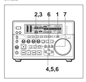
Press the COUNTER SELECT button to light the time data type indicator "TC" or "U-BIT."
